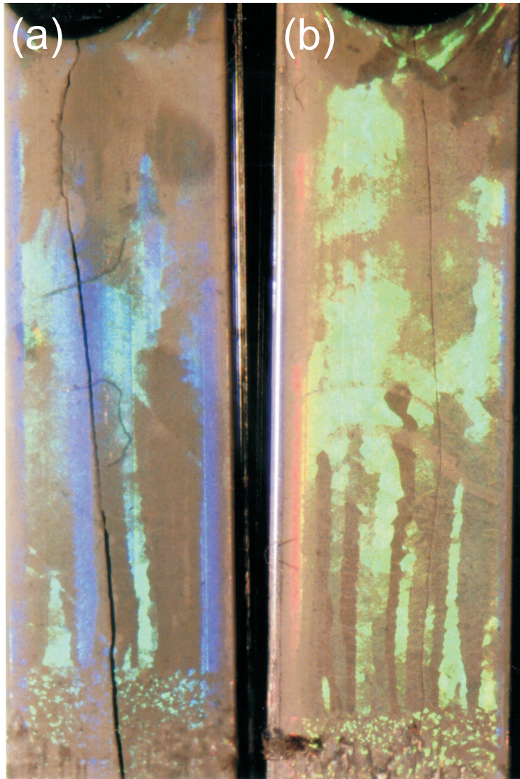
FIGURE 3.4: Optical micrograph of two opals (a) and (b), that both consist of polystyrene spheres with radius r = 460 nm. Colorful blue and green reflections are apparent, resulting from optical Bragg diffraction. At the bottom of the opals many small crystallites are present, caused by fast crystallization by centrifugation. The upper part of the samples consist of large crystals, due to slow crystallization. A long vertical crack is present in both opals, caused during drying from colloidal crystal to opal.
